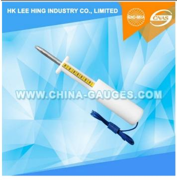
Rigid Test Finger Probe of IRAM 4220-1 / IEC 61032 / IEC 60335
