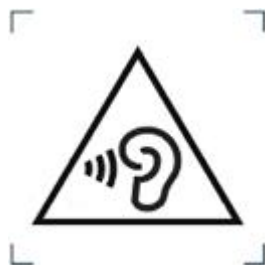
Figure Z1 – Warning label (IEC 60417-6044)
